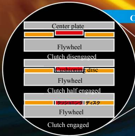
Red disc indicates the cushioning disc
